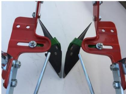
When mounted side by side, the blades work together and direct soil away to create a furrow for planting crops like potatoes or leeks. In this orientation, the
