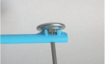
To calibrate, expose the thermometer to a known temperature. This can be done by filling an insulated container such as a travel mug with ice and then filling with water. Wait a couple minutes then stir the ice and insert the thermometer. Wait another minute and then turn the nut relative to the face until it reads 32°F/0°C. It will now be calibrated.
