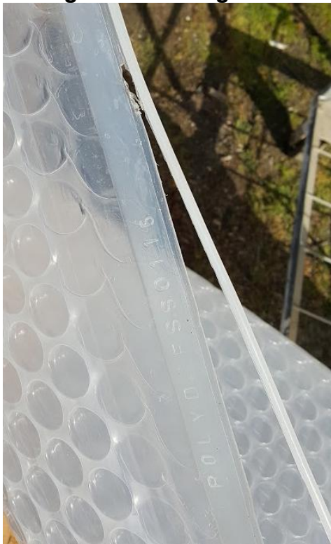
Damage from misaligned connectors.
