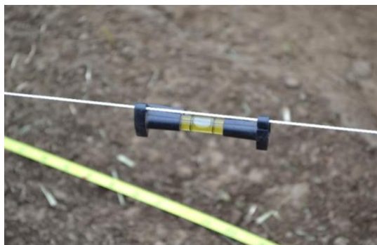
Figure 3: Mason line and line level.
