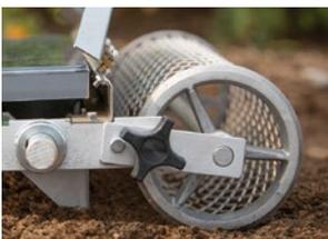
Open wheel ends for easily cleaning out the wheel cage
