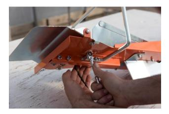
2. Fasten the tray platform to the body with the 2 carriage bolts provided, using the 13mm wrench.
