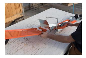
3. Secure the adjustable wheel stem to the head of the tray platform with the 2 included carriage bolts. Make sure to use the square hole to accept the carriage bolt, with the washers on the opposite side (see inset below).
