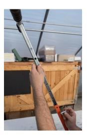
5. To adjust the planting depth you can raise and lower the height adjustment, shown below. To plant deeper, use the lowest setting. To plant shallower, raise the adjustment. Experiment to see what works best for your soil conditions. Remove the latch pin completely to make this adjustment easier.
