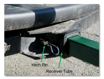
STEP 2: Slide the end with the large predrilled hole into the receiver tube on your vehicle. Secure with any standard hitch pin or large bolt.
