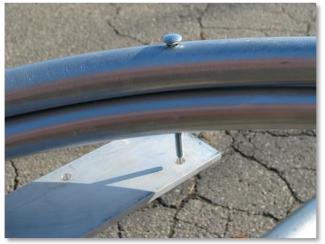
**STEP 5:** Use the single hole nearest the vehicle for either bender; and one of the other holes on the opposite end depending on which bender you have.
