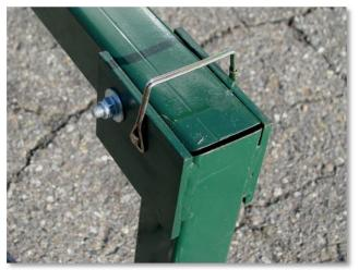
STEP 1: Remove wire-lock clevis pin from green hinged portion of mount, rotate support arms so they are at right-angles to each other, and secure with wire-lock clevis pin.
