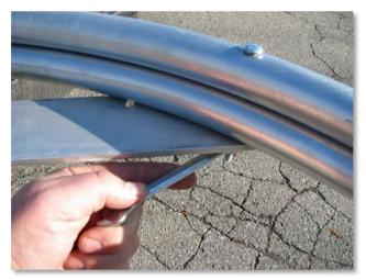
**STEP 6:** Using a  $^{7}/_{16}$ " wrench, secure either 4- or 6-foot Quick Hoops Bender using the two  $\frac{1}{4}$ " x 4- $\frac{1}{2}$ " carriage bolts, nuts, and washers.
