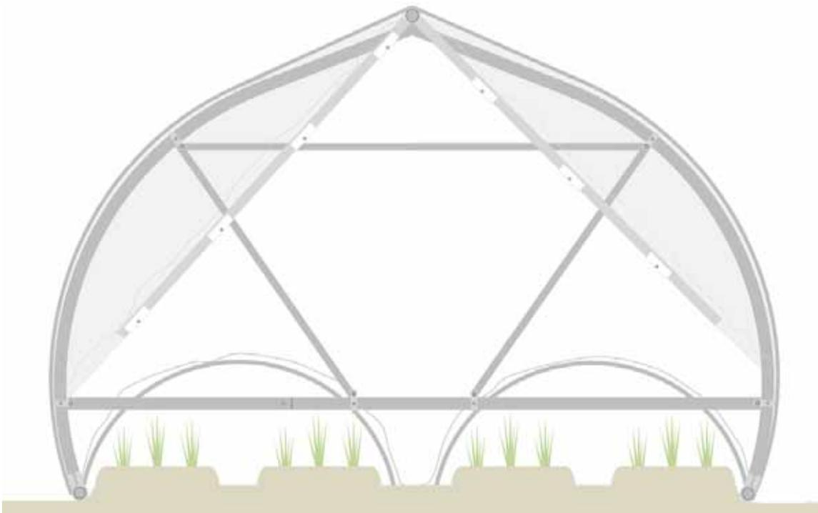
16. **Roll-up Sides:** There are a couple options here. You can choose low cost manual roll-ups that require manually rolling up each side of each module individually, or you can choose hand crank roll-ups that allow you to roll up the entire side of the tunnel all at once.
