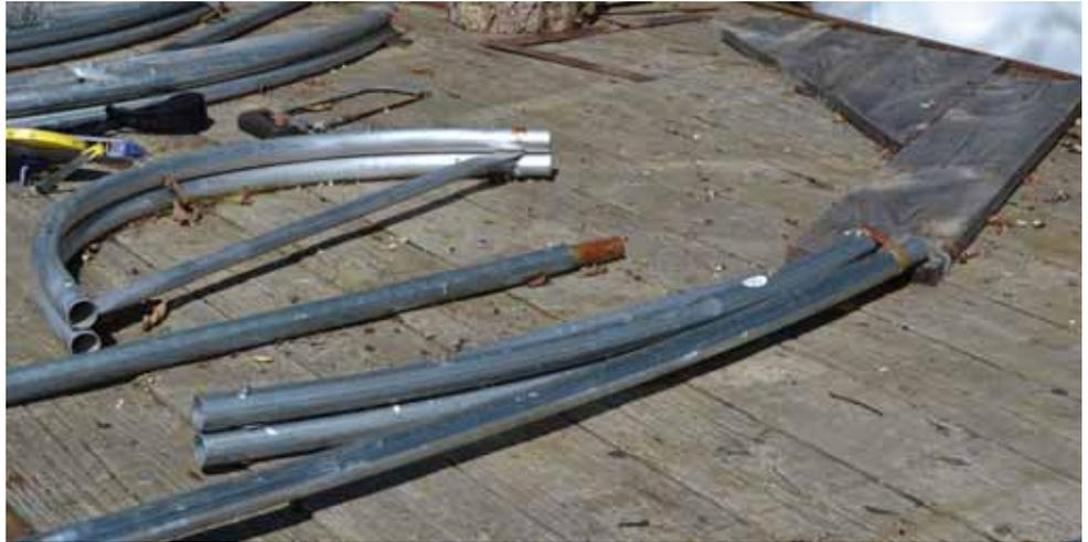
Wherever the bender is mounted, it is important to have both enough room to accommodate the in-feed and out-feed of pipe, as well as some type of support at the out-feed end about 3/4" above the mounting surface. This will prevent 'corkscrewing' and ensure that the hoophouse bows created are in a single plane.
