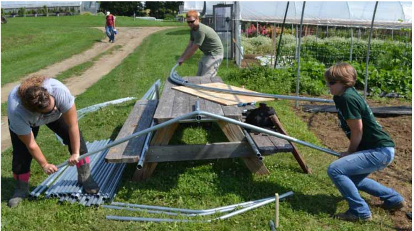
Both the curved bender and the Peak Jig may be mounted to any solid surface, such as a workbench, a picnic table, hay wagon, etc. They may be lag-screwed or thru-bolted into place. 5/16" mounting holes are provided on them and the screws, bolts, etc. to mount them are also included. By securing the bender and jig fixed positions, and pulling the tubing around them the operators can maintain precise control of the tubing being bent.
