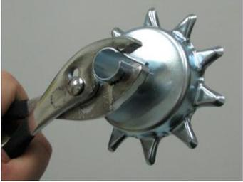
7. For proper operation, the wheel ferrules must grip the shaft firmly without slipping. If wheel ferrules do not grip tightly enough, they may be adjusted by gently compressing with a pair of round-jaw pliers until the ferrule hole becomes slightly smaller than the shaft. See left. **Be careful to not over-compress.**
