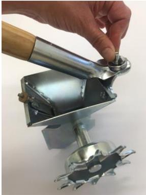
**Seeding Depth:** The seeding depth is determined by the angle at which you hold the handle in relation to the ground. Holding the handle lower to the ground will sow seeds deeper in the soil and raising the handle will sow seeds closer to the soil surface. This will take some practice to consistently sow at the same depth.
