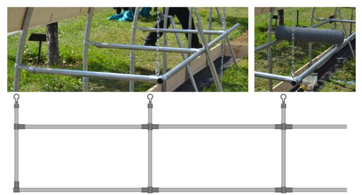
9. Attach the 2 longer rear rails (B) and 1 shorter rear rail (C) to the 3 longer cross rails (D) using 1 end rail clamp (I) and 2 line rail clamps (H) per this diagram. Position the rear rails using the shorter cross rails (E) as spacers between the front and rear rails. Clamp everything in place, and adjust as necessary, using the wire mesh roll to spot check shelf width. When you are satisfied that everything is aligned correctly, install tech screws in the smaller holes of the clamps.
