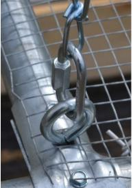
hex bolt and  $\frac{3}{8}$ " nylock hex nut. Loosen each brace band by holding the hook and turning the frame until each is extended about  $\frac{2}{3}$  of its full reach.
