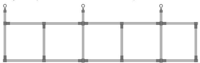
10. Attach the 3 shorter cross rails (E) using 6 end rail clamps (I) per this diagram by clamping and installing tech screws.
