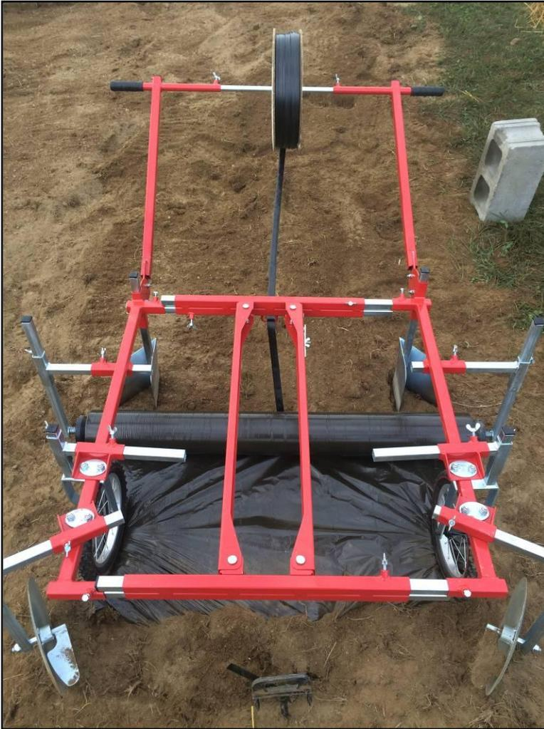
2) Position the mulch layer at the beginning of the first row to be covered and pull it forward until the trench made by the plows lines up with the rear part of the frame.
