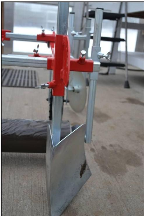
8) To set up your spindles properly you will need a roll of mulch. Start by centering the roll so that at least 3 inches of the roll extends past the inside edge of the front plows. Adjust the height of the spindles so that the roll of mulch is about 4 inches above the bottom point of the plows (ground level).
