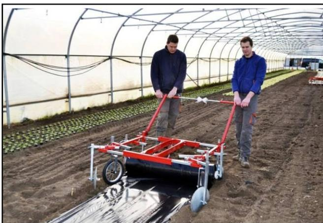
11) Two people are required to pull the mulch layer; we found that setting the handles at hip height offered the most ergonomic use. When you are ready to move your mulch layer to the field, you can lower the press wheels as low as they will go and align them with the frame so that they can be used for transport. If there is the need for frequent longer distance transportation, we have special transport wheels available that are more durable than the press wheels that come with the mulch layer.
