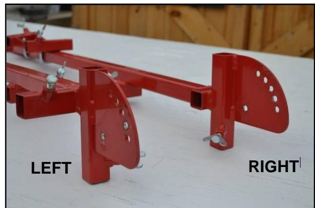
6) After mounting the toolbars to the central frame, you are ready to begin adding the toolbar implements. **We recommend that you set up your mulch layer on a hard flat surface; this will help get things set up squarely.**
