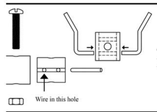
**4.** Insert wire ends into plug hole where arrow shows.
