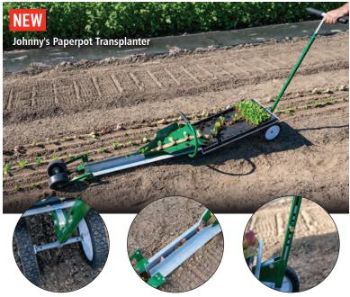
Adjustable front axle for optional tighter spacing and improved productivity
