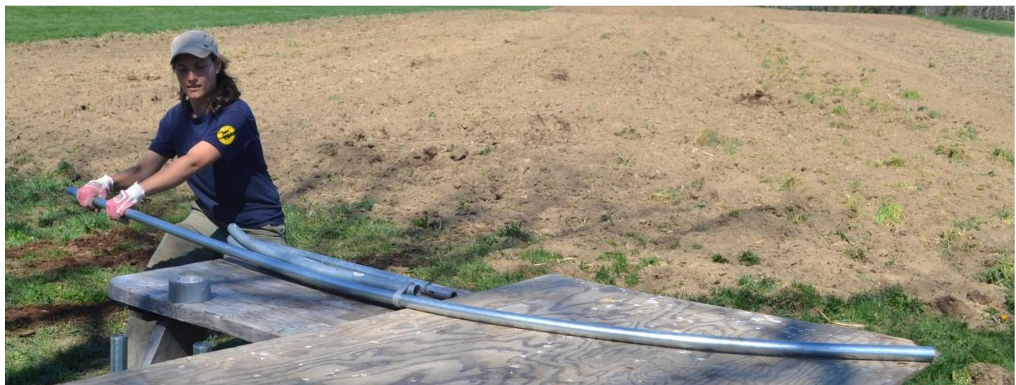
The Quick Hoops™ High Tunnel Bender may be mounted to any solid surface, such as a workbench, a picnic table, hay wagon, etc. It may be lag-screwed or thru-bolted into place.  $\frac{5}{16}$ " mounting holes are provided on the bender and the hardware to mount it are also included. By securing the bender in a fixed position, and pulling the tubing around the bender, the operator can maintain precise control of the tubing being bent.
