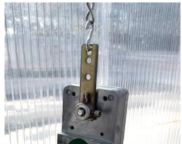
Figure 7: Attaching the S-hook and chain to the mounting arm.
