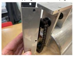
**3.** Loosen and remove lock collar at end of shaft with 3.5 mm Allen wrench (*Figure 3*).
