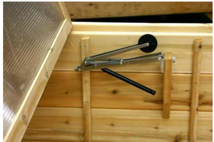
**Univent Adjustment:** The only adjustment is the threading in or out of the cylinder. With the temperature cool enough so you'd like the door to be closed, adjust the cylinder so the wheel just touches the door and will start to open it as soon as it expands.
