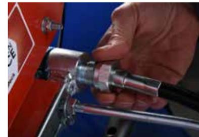
(21) Then screw the lower nut of the hose onto the angle transmission of the pick-up reel.
