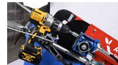
(25) Adjust the positioning of the part that controls the trigger of the drill and tighten the drill using the plastic toggle latch
