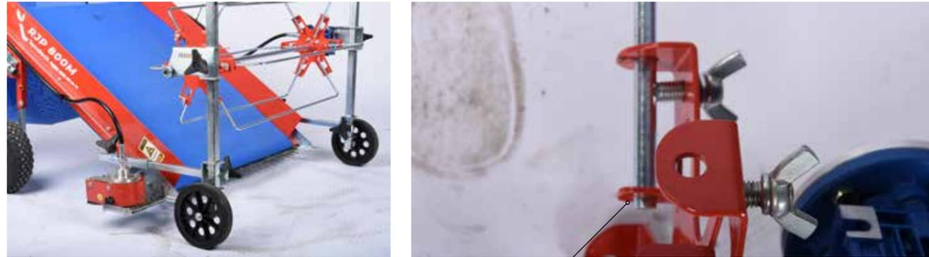
The bar is assembled in both holes
