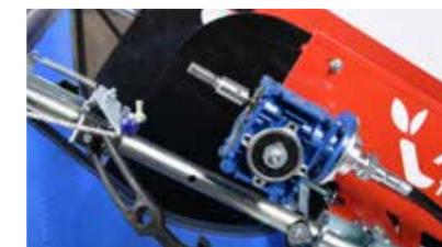
(23) Fit the drill onto the arm of the machine by pushing the chuck onto the hexagonal shaft.
