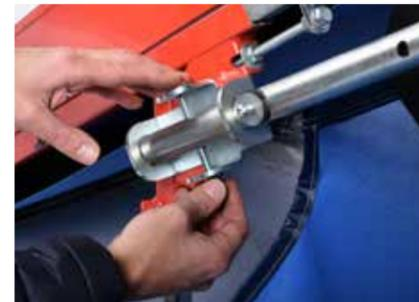
(14) Connect the horizontal tube of the wheel to the vertical tube of the pick-up reel: the star screw must be on the side opposite the wheel.
