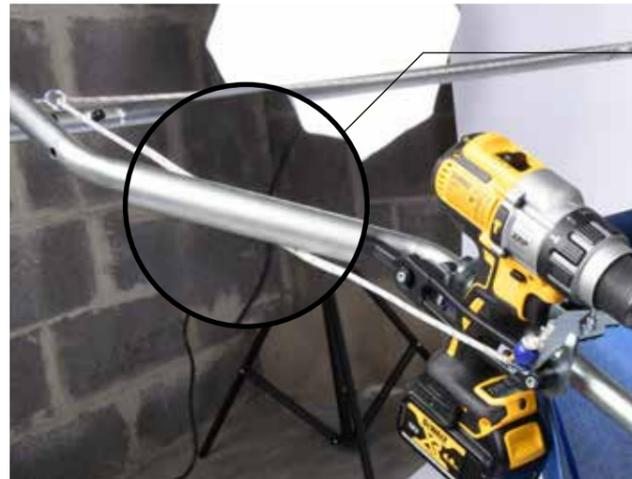
(27) Check that the control cord passes under the right half-handle so that it can properly activate the trigger of the combi-drill.
