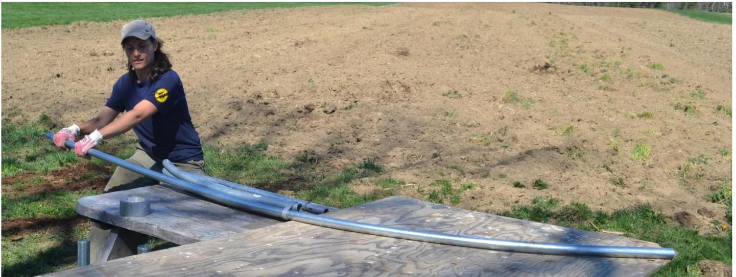
The Quick Hoops™ High Tunnel Bender may be mounted to any solid surface, such as a workbench, a picnic table, hay wagon, etc. It may be lag-screwed or thru-bolted into place. <sup>5</sup>/<sub>16</sub>" mounting holes are provided on the bender and the hardware to mount it are also included. By securing the bender in a fixed position, and pulling the tubing around the bender, the operator can maintain precise control of the tubing being bent.
