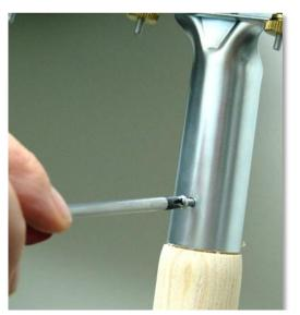
3. Using a #1 Phillips screwdriver, secure the seeder body onto the handle with the #4 x 1/2-inch wood screw provided.
