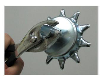
7. For proper operation, the wheel ferrules must grip the shaft firmly without slippage. Also, a slight gap between the wheel ferrules and the body of the seeder must be present so the wheels and axle will turn freely without friction.
