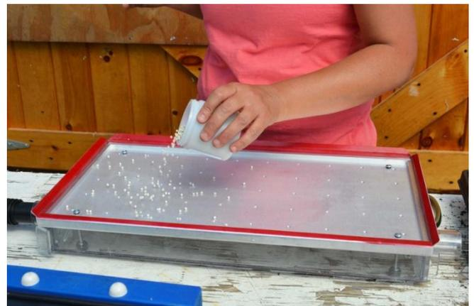
3. **Valve adjustments:** Note two generalities: Small, light seeds require very little air flow and lower vacuum pressure in order to be attracted to the seed holes (i.e.: bypass valve more open). Conversely, larger, heavier seeds require greater air flow and higher vacuum pressure in to defy gravity (i.e.: bypass valve more closed).
