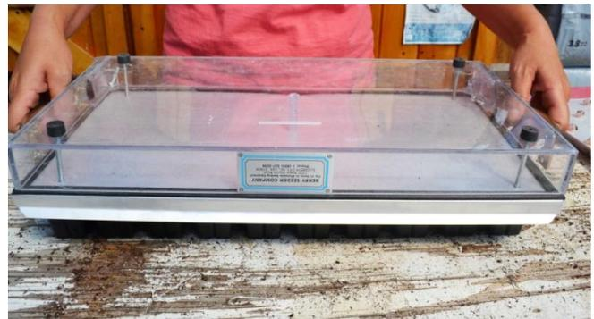
**9. Releasing the seed:** Open the on/off valve. Tap the back of the seeder body with your hands. Lift the seeder body off the growing tray. Cover and water the seeds as you normally would. Repeat steps 2 through 6 for subsequent trays.
