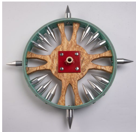
12" Spacing Dibbles on the 4 "corners"
