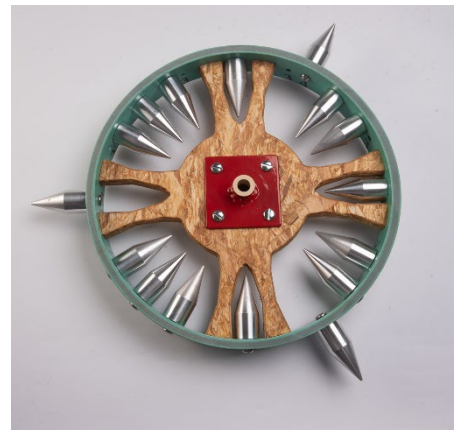
15" Spacing Dibbles on every 4 th 4-3 hole
