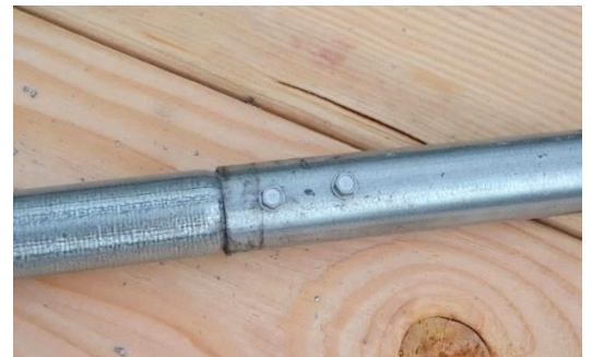
Figure 6: Tek screws securing bow assembly.
