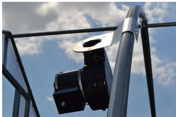
Figure 36: Bracket and blower motor mounted to the bow.
