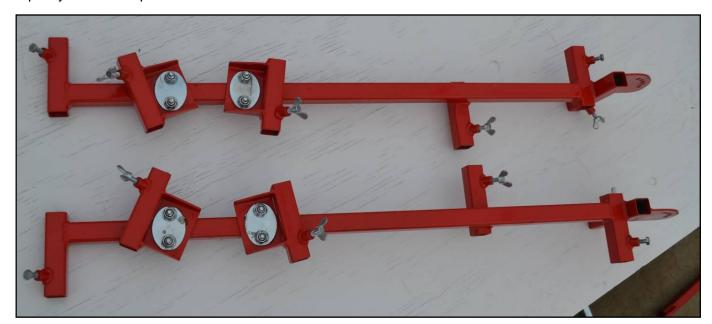
5) Before mounting the toolbars, reference the diagram that was included with your mulch layer. Notice that the right side of the mulch layer has tool arms that look like a T and the left side has arms that look like an L (below left). This is to compensate for the frame extension arms being stacked on top of each other. The toolbars themselves are similarly altered (below).
