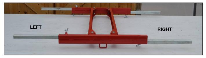
4) Locate the right and left toolbars (shown below). The brackets for the press wheels and spindles should match up pretty closely when set side-by-side. In our trials we noticed that if the lock nuts on these were not tightened sufficiently, they had a tendency to move during use, which could negatively affect the quality of the end-product.
