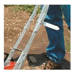
3. Determine the desired height of the handle. Attach the stock handle to the extension bars using the nuts and the larger bolts that came with the handle extension kit. These bolts are longer, so that if you only raise the handle 1 notch, they can pass through the 3 overlapping aluminum bars.
