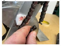
3. Remove gear sprocket locking pin. Heat both sides of the pin to break the lock tight, then drive out the pin with a hammer and pin driver tool. (Figure 3.)
