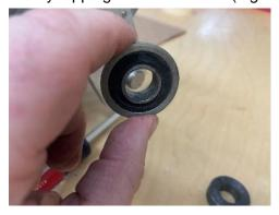
**2.** Remove bearing by prying evenly with a standard screwdriver (*Figure* 2).
