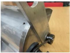
**3.** Install new bearing by sliding it over the shaft and carefully tapping it back into hole (*Figure 3*).
