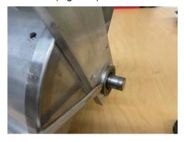
**4.** Reinstall lock collar by sliding it over the shaft and tightening the set screw (*Figure 4*).
