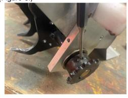
**4.** Remove gear sprocket by loosening the set screws, removing the two set screws, and sliding the sprocket off of the shaft (*Figure 4*).
