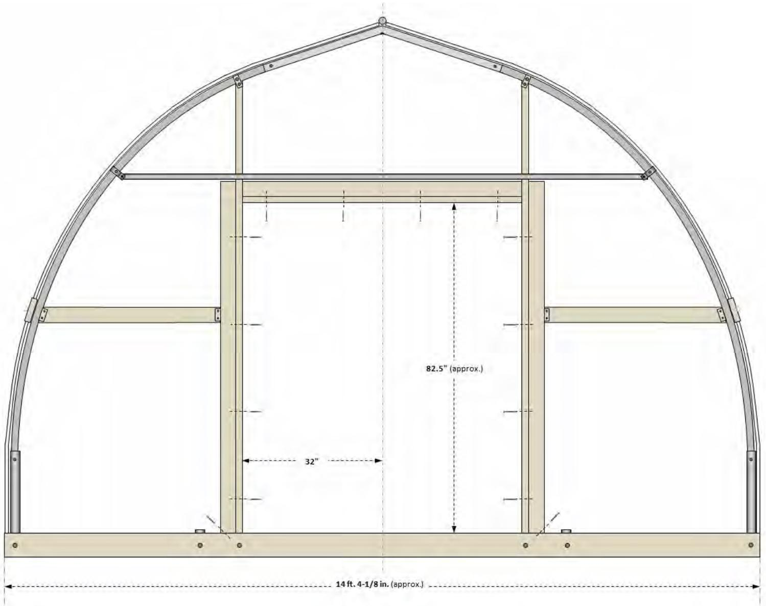
j. Cut two more pieces of 2" x 4" to a length of 64". Place one at the top of the door opening so that the wide edge is facing the end of the tunnel. Secure at each end with a couple 3" bugle head wood screws. Place the second one under the first with its narrow edge facing out and flush with the outside edges of the door frame. Secure at each end with a couple 3" bugle head wood screws, then secure the second board to the first with four more 3" bugle head wood screws.
