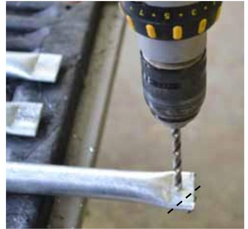
2. With a 5/16" drill bit (cobalt bits work best), drill through the center of the flattened area on each tie.
