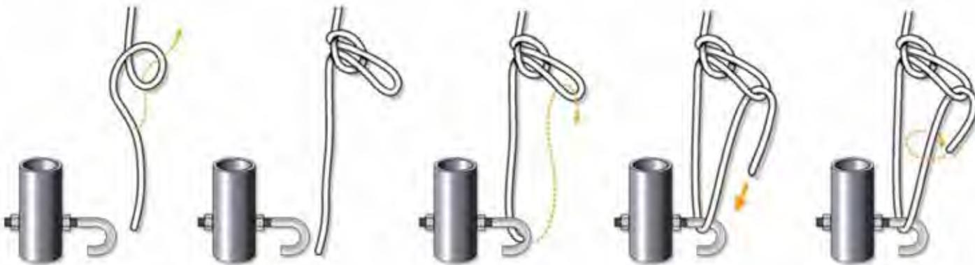
*A Trucker's Hitch is used to tension lacing on the roll-up sides.*
