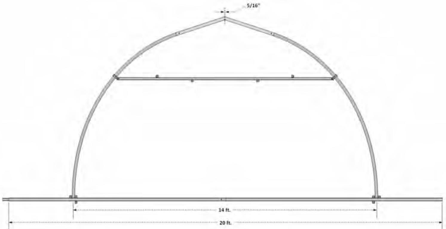
1. Use two pieces of top-rail as part of the jig for assembling the bows. On a flat area of ground, arrange some small stakes to create the jig around the top-rail as shown above.
