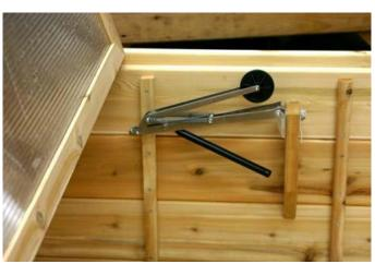
**Univent Adjustment:** The only adjustment is the threading in or out of the cylinder. With the temperature cool enough so you'd like the door to be closed, adjust the cylinder so the wheel just touches the door and will start to open it as soon as it expands.
