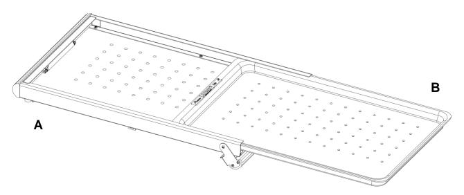
Drop seeder tray with 72 3mm holes (B) comes pre-installed in the drop seeder frame (A).
