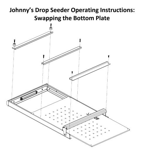
To change cell pattern, you will need to swap both the polycarbonate bottom plate and the drop seeder tray (check Johnnyseeds.com for additional plate and tray options). To swap the bottom plate:
