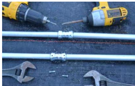
Figure 43: EMT connected with compression coupling.
